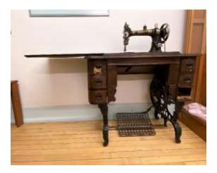
A sewing machine like this is powered by the operator by means of the foot pedal. This model of sewing machine was produced from the 1880's-1960's.
