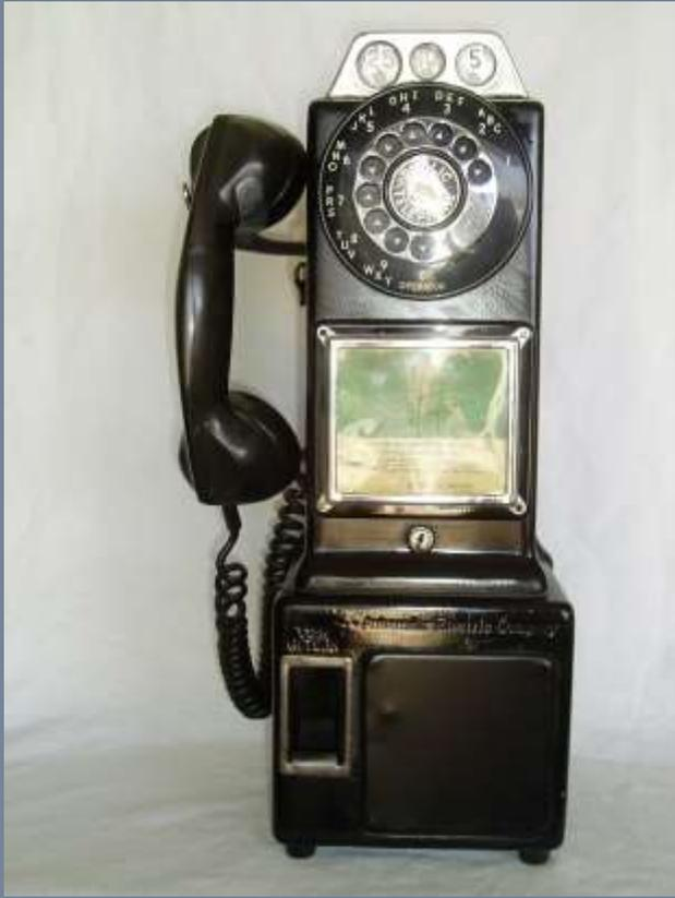
In 1898, the Western Electric No. 5 Coin Collector, the first automatic "prepay" station, went into use in Chicago. The depositing of coins before placing a call would gradually become the norm in pay phones until the introduction of "dial tone first" service in 1966.
