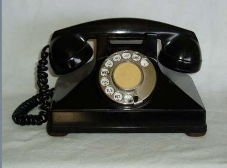
This is a 1930's Kellogg Master phone 1000 "Red Bar", so named because the hook switch under the handset is a red plastic bar. This is one of the very hard to find metal bodied ones and represents one of the last of the "Master phone" series. This is a heavily Art Deco influenced series of designs. The name is the model name of the particular handset found on all these models. This one has a new black powder-coat finish.
