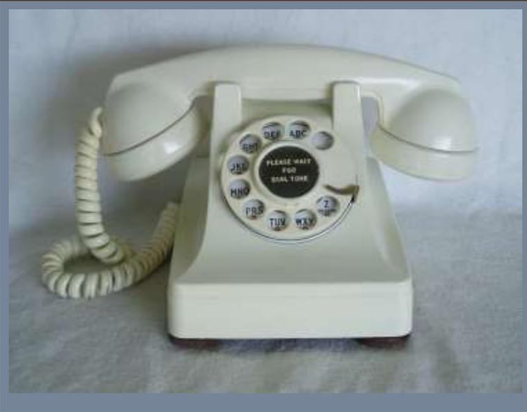
This is the baby boomer phone of the 40's and 50's. It is a Western Electric original and it's Bakelite handset is classic and heavy. The bases were either steel or plastic and the true bell ringer brings back memories of old times. This is a common phone and a true classic made mostly in black. A white one is rare!
