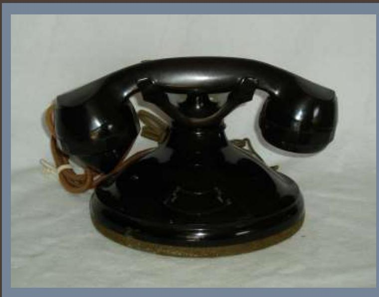
The HTF "Real Phone" was put out by the American Automatic Electric Sales Co. The diameter of the base is 5 1/4" the handset is 7 1/8"L and is 4"H. This is a very unusual early Telephone that was used in many homes during the first half of the 20th century. The brass plate on the front reads "Real Phone American Automatic Electric Sales Co. Chicago, U.S.A. Pat. 1,976,729."
