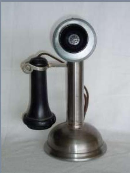
This is a Stromberg-Carlson style candlestick telephone called the "Tapered Shaft Desk Set." This phone was nicknamed "oilcan" because of its odd shape.
