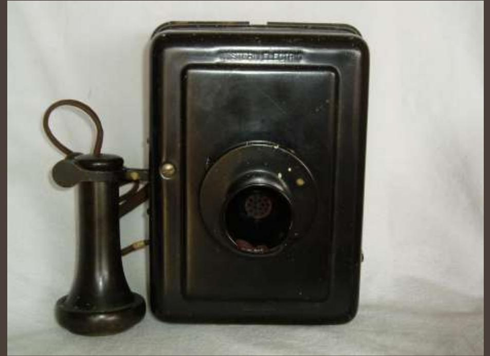
These are compact style Western Electric wall phones. The phones were initially small wood models and shortly thereafter of copper plated sheet metal composition having two coats of black enamel paint. Western Electric compact wall phones, although plain, were highly desirable, as they require minimal wall space for display.
