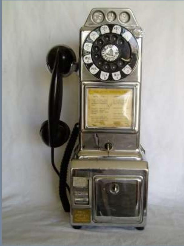
The 50A coin collector, went into production in 1911. By the end of 1912, 25,000 of these coin telephones had been ordered for New York City alone. The 50A model had three coin slots--for nickels, dimes and quarters --and was a "prepay" machine. The basic design, though often modified, was so practical and reliable it remained in production until 1964.
